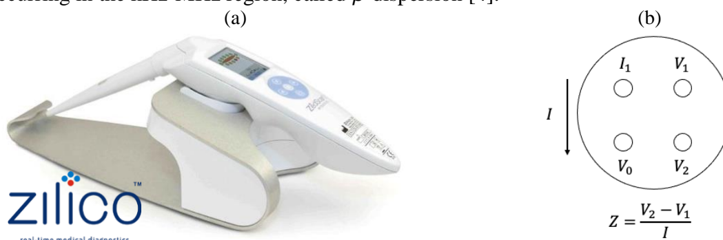
Figure 1 Electrical Impedance Spectroscopy device: (a) ZedScan™ [5], (b) tip of the tetrapolar probe showing the principle of the measurement, a known current I flows between the active electrodes ( I_1 and V_0 ) while the passive electrodes ( V_1 and V_2 ) capture the potential difference at different frequencies
